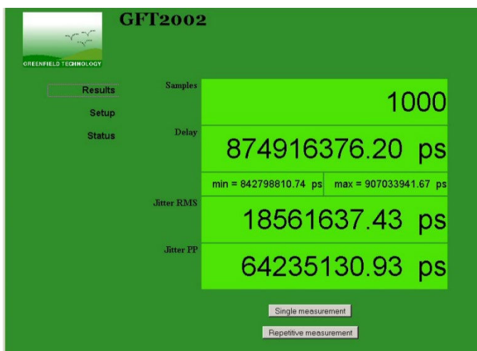
GFT2002 control panel web page
